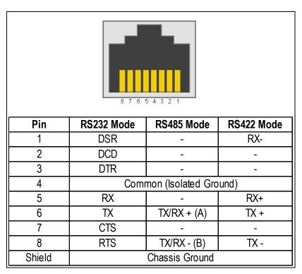
Figure 11: RJ45 Port pin-out
